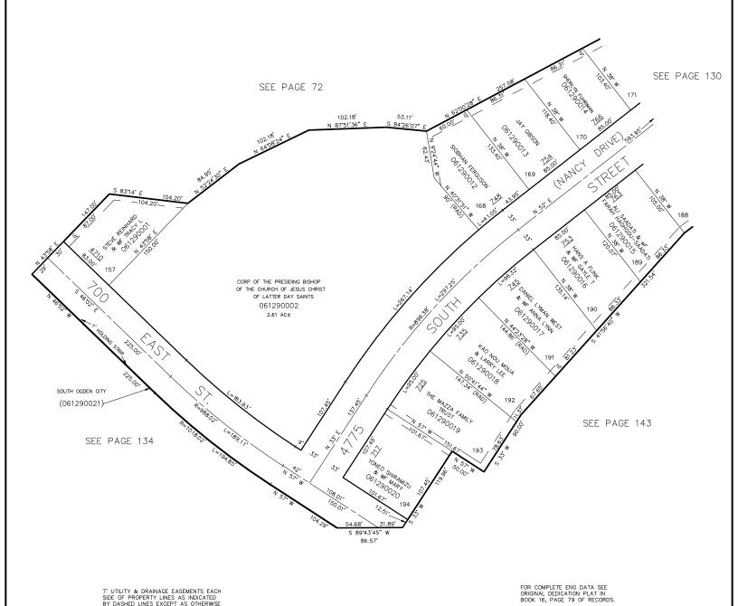
7' UTILITY & DRAINAGE EASEMENTS EACH SIDE OF PROPERTY LINES AS INDICATED BY DASHED LINES EXCEPT AS OTHERWISE SHOWN.
